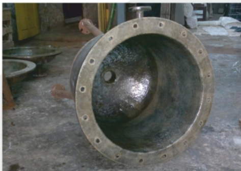
FRP Lined Equipments
